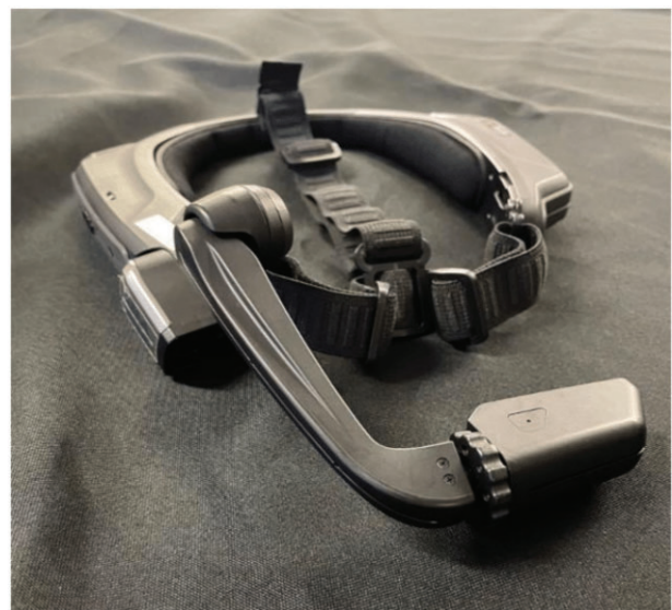
Figure 1. Stryker IRIS headset to allow video and audio link between surgeon and audience.
