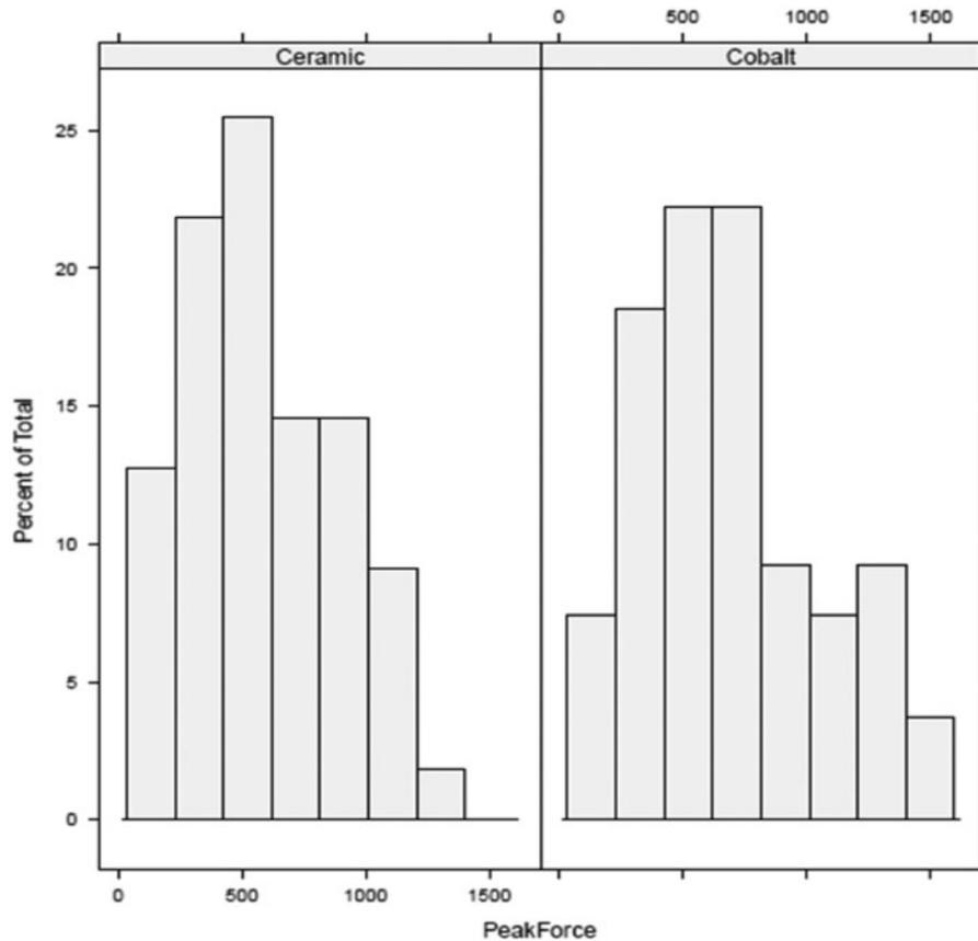
**Figure 2.** Histogram of each surgeon's effective coupling force (lbF) for cobalt and ceramic heads.
