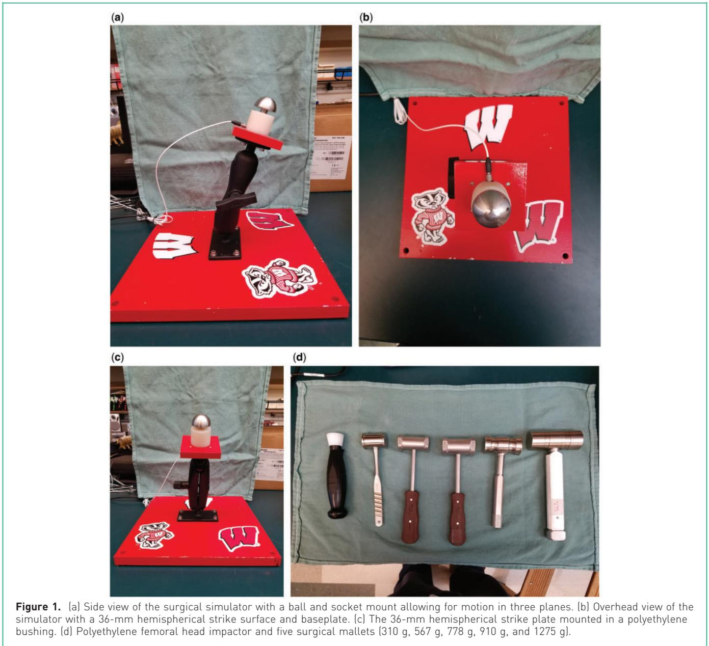
**Figure 1.** (a) Side view of the surgical simulator with a ball and socket mount allowing for motion in three planes. (b) Overhead view of the simulator with a 36-mm hemispherical strike surface and baseplate. (c) The 36-mm hemispherical strike plate mounted in a polyethylene bushing. (d) Polyethylene femoral head impactor and five surgical mallets [310 g, 567 g, 778 g, 910 g, and 1275 g].
