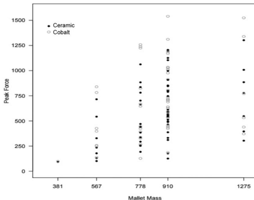
**Figure 3.** Scatter plot of the effective coupling force (lbF) versus mallet mass with 1, 2, 3, and 4 kN thresholds identified.
