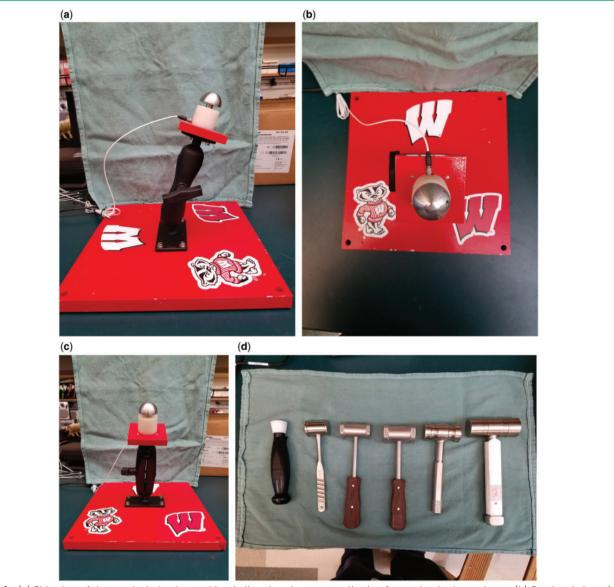
**Figure 1.** (a) Side view of the surgical simulator with a ball and socket mount allowing for motion in three planes. (b) Overhead view of the simulator with a 36-mm hemispherical strike surface and baseplate. (c) The 36-mm hemispherical strike plate mounted in a polyethylene bushing. (d) Polyethylene femoral head impactor and five surgical mallets (310 g, 567 g, 778 g, 910 g, and 1275 g).
