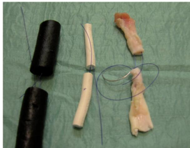
**Figure 1.** Tendon simulator models. Left to right: liquorice, sealant, porcine.
